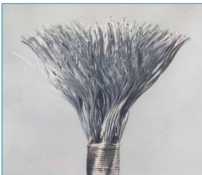
Incorrectly Broomed Wire Rope
