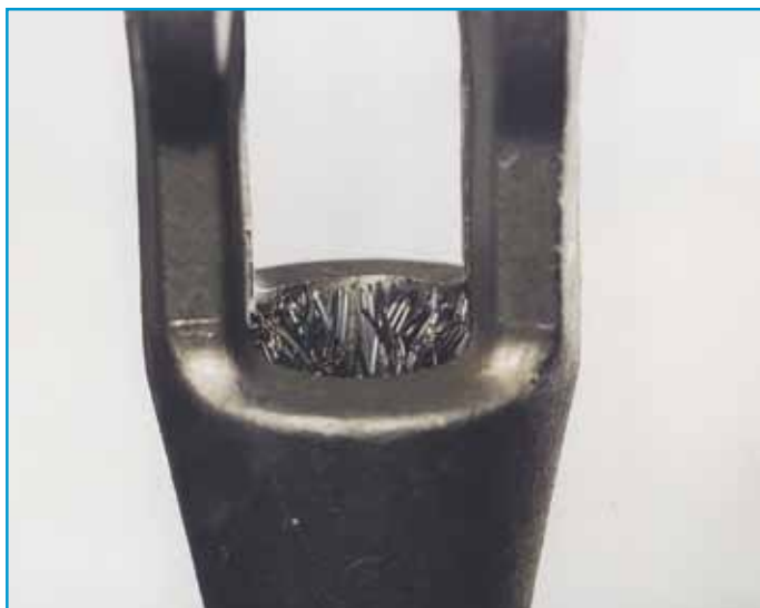
Properly positioned broom with the wire ends protruding slightly (Fig 3)
