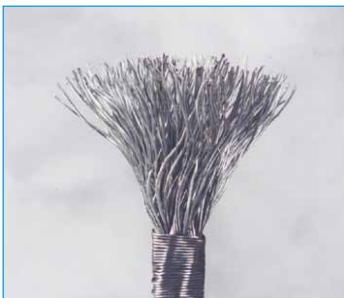
Properly Broomed Wire Rope (Fig 2)
