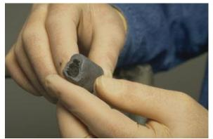
1. Cut off the desired amount to be used. Peel off protective wrap.
