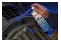
Cold Galvanising Spray is a unique combination of zinc powders and resins, formulated to form a high performance zinc-rich coating that actively fights rust and corrosion by its galvanic properties. Ferrous metals are protected by the sacrificial action, even when scratched or damaged. Zinc becomes the anode which is attacked by corrosion and the base metal the cathode. A film of water-insoluble zinc oxide is formed, which stops rust and corrosion.
